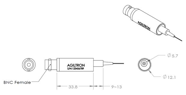
dimensions tolerance to be +/-0.2mm
